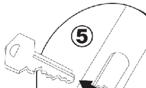
5 Practice a light pressure over the bow and take the key off
